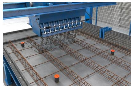
Install steel reinforcement and concrete
